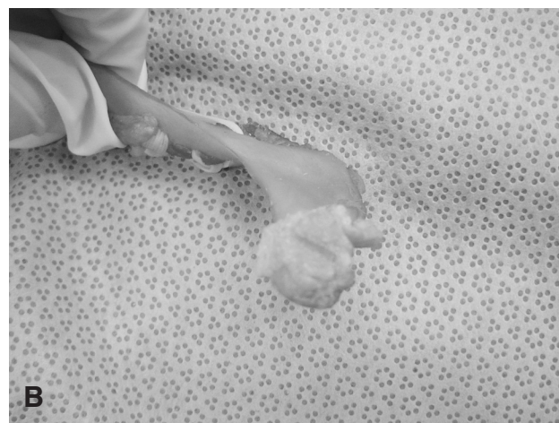
Figure 4 A, Failure of the bone plug specimen on the MTS machine. B, Area of suture cut out in the bone plug.
